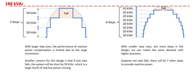
Additionally, by having smaller steps the VARIVAR can match the load profile better and is more accurate in its compensation, keeping your system closer to Unity. Another advantage to having three times the number of capacitors is that if one fails the effect on performance is minimal.
