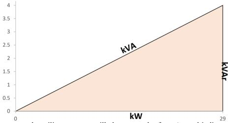
On the left is a power triangle, which illustrates the relationship between each power. As you can see, the kVA is just a result of a kVAr and kW value. Most utility companies charge a flat kVA capacity, which is the expected power distributed and returned. However, if the load overdraws this dedicated
