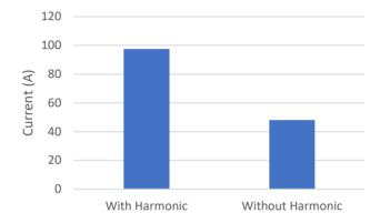
Graph above shows the difference in current between the peak current with harmonics and the without harmonics. It appears that the filtered harmonic current is higher due to some resonance in the harmonic current.
