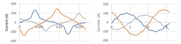
Suppose we remove the small amounts of harmonic we measured, the resulting waveforms (on the right) would resemble near perfect sine waves.
