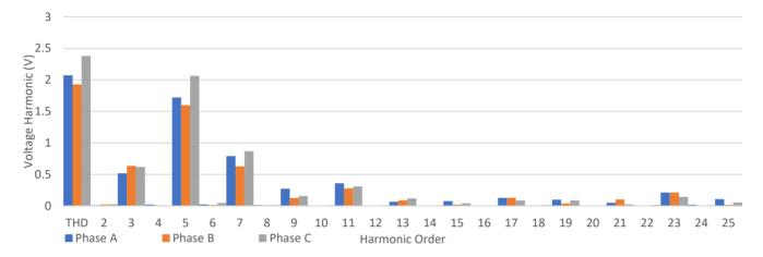
Displayed above is the harmonic content measured with your system. The measure harmonics are within IEEE 519 standards and should not harm the operation and its equipment.
