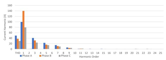
As you can see, the 3rd, 5th, 7th and 9th harmonic is high relative to the other voltage harmonics. Having high voltage harmonics can cause extra load consumption since the peak voltage with harmonics will be greater. Another common harmonic issue is that it will cause voltage unbalance between the phases. The motor's life span will reduce as a result due to either overloading or irregular voltage signals.
