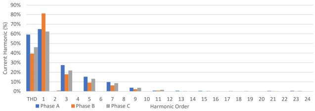
The graph above shows the current value as a percent of the total current measured, which in this case is 97.5A. Again, as you can see, the 3rd, 5th, 7th and 9th harmonic is the highest harmonic in the system.
