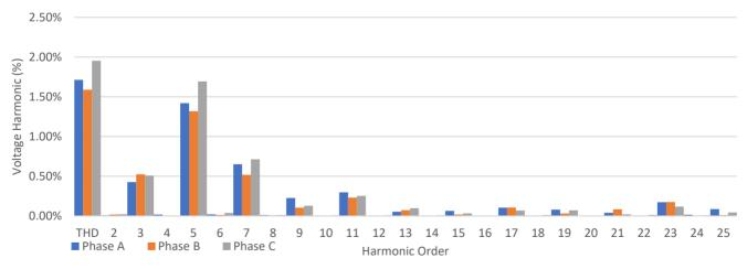
The graph above shows the voltage value as a percent of the total voltage measured, which in this case is 121.13V. Again, as you can see, there are no dangerous harmonics within your system.
