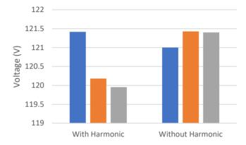
The graph above shows the voltage per phase. As you can see, the voltage levels are more balanced due to correcting the voltage harmonics. In fact, this is a direct cause in reducing the current harmonics, which extends the life of your motors and other electronic equipment.
