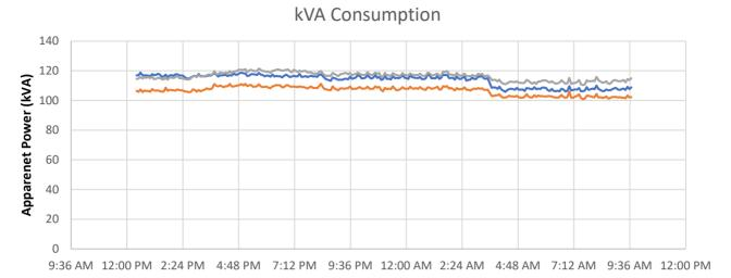
The total kVA consumed by the load is 337 kVA. This value represents to total power flowing, both power used by the load and absorbed/returned. In other words, kVA is the result of both the kVAr and kW. This relationship can be further explained with a power triangle.
