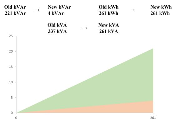
As shown above, there is a change in the power triangle. The green represents the old power triangle with its kVAr, kW, and kVA. The orange is the new power triangle, noticeably smaller than the previous power triangle. This illustration shows the reduction of energy consumed by the system simply due to changes in the power factor.
