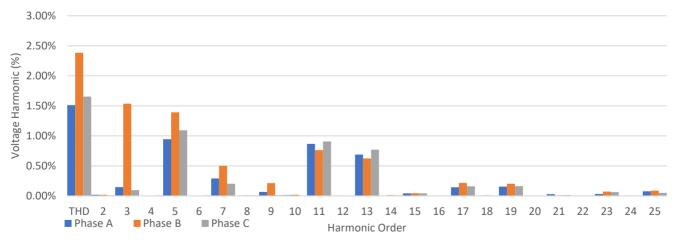
The graph above shows the voltage value as a percent of the total voltage measured, which in this case is 285.76V. Again, as you can see, there are no dangerous harmonics within your system.
