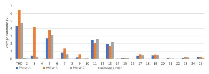
Displayed above is the harmonic content measured with your system. The measure harmonics are within IEEE 519 standards and should not harm the operation and its equipment.
