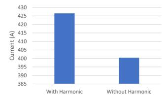
Graph above shows the difference in current between the peak current with harmonics and the without harmonics. It appears that the filtered harmonic has a lower current due to the reduction in current harmonics.
