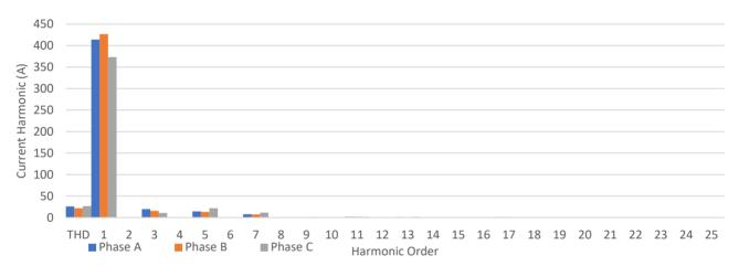
Displayed above is the harmonic content measured with your system. The measure harmonics are within IEEE 519 standards and should not harm the operation and its equipment.
