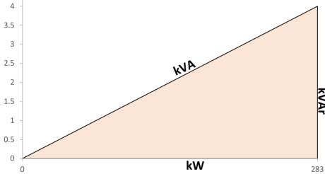
On the left is a power triangle, which illustrates the relationship between each power. As you can see, the kVA is just a result of a kVAr and kW value. Most utility companies charge a flat kVA capacity, which is the expected power distributed and returned. However, if the load overdraws this dedicated
