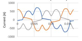
to the left is observed. This is the typical waveform of a six-pulse VFD setup. When we investigated the distribution at the MCC of the water park, our theory was confirmed by the sightings of Siemens VFDs. From the looks of it, these VFDs already have a DC link choke installed to limit the current harmonics from 70% to 30%, however, this number is still concerning for the
