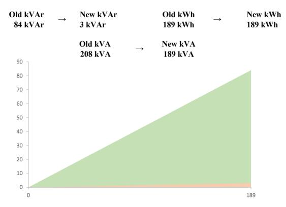
As shown above, there is a change in the power triangle. The green represents the old power triangle with its kVAr, kW, and kVA. The orange is the new power triangle, noticeably smaller than the previous power triangle. This illustration shows the reduction of energy consumed by the system simply due to changes in the power factor.
