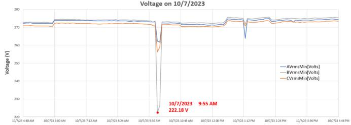
As shown in the graph above, there was a voltage sage on Saturday, October 7, 2023. The event was momentary and was restored within 10 minutes. We suspect this voltage drop to be the result of a large current load being turn on. This could be the result of multiple large loads simultaneously being switched on.
