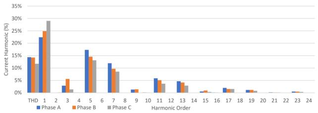
The graph above shows the current value as a percent of the total current measured, which in this case is 257.04A. Again, as you can see, the 3rd, 5th, 7th, 9th, 11th, 13th, 15th, 17th, 19th, 21st, 23rd and 25th harmonic is the highest harmonic in the system.
