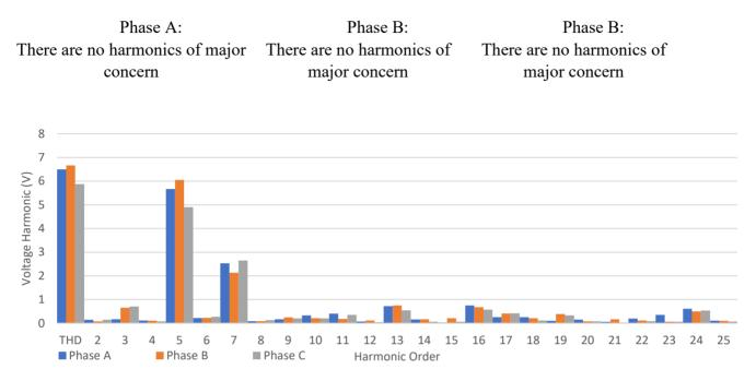
Displayed above is the harmonic content measured with your system. The measure harmonics are within IEEE 519 standards and should not harm the operation and its equipment.
