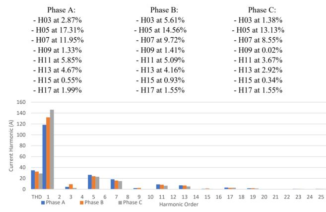
As you can see, the 3rd, 5th, 7th, 9th, 11th, 13th, 15th, 17th, 19th, 21st, 23rd and 25th harmonic is high relative to the other voltage harmonics. Having high voltage harmonics can cause extra load consumption since the peak voltage with harmonics will be greater. Another common harmonic issue is that it will cause voltage unbalance between the phases. The motor's life span will reduce as a result due to either overloading or irregular voltage signals.
