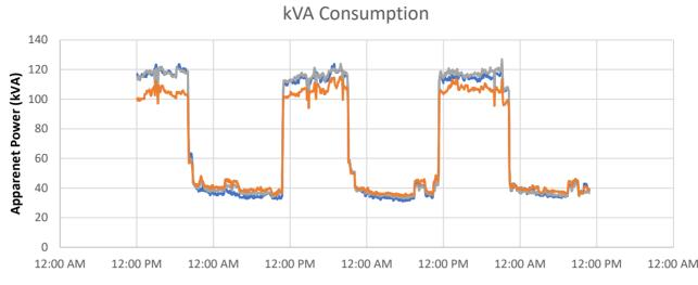
The total kVA consumed by the load is 208 kVA. This value represents to total power flowing, both power used by the load and absorbed/returned. In other words, kVA is the result of both the kVAr and kW. This relationship can be further explained with a power triangle.
