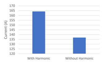
Graph above shows the difference in current between the peak current with harmonics and the without harmonics. It appears that the filtered harmonic has a lower current due to the reduction in current harmonics.
