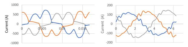
Suppose we remove the small amounts of harmonic we measured, the resulting waveforms (on the right) would resemble near perfect sine waves.
