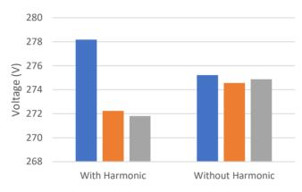
The graph above shows the voltage per phase. As you can see, the voltage levels are more balanced due to correcting the voltage harmonics. In fact, this is a direct cause in reducing the current harmonics, which extends the life of your motors and other electronic equipment.
