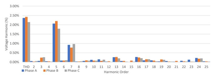
The graph above shows the voltage value as a percent of the total voltage measured, which in this case is 274.49V. Again, as you can see, there are no dangerous harmonics within your system.
