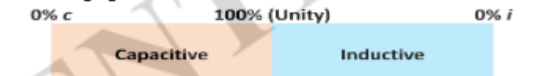
Figure 1. Centered down the middle is power factor unity – where power is ideally utilized at 100% efficiency. For inductive loads, if it becomes too capacitive, the system is deemed leading. Leading power factor can cause equipment damage due to voltage exceeding the capacity of the equipment.
